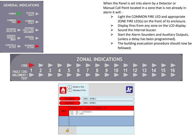
The LCD gives all the alarm information, such as the time & date of the alarm, the address, the device type, the device label, and the zone it is allocated to.
