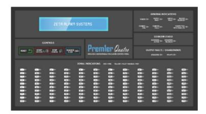
If the repeater is connected and communicating to the Quatro panel correctly, the "CONNECTION WITH PANEL ON" digital LED will be GREEN. If there is a connection issue, this digital LED will be shown in YELLOW. If connection problems do arise then make sure the system settings are correct.
