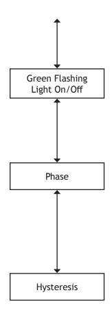
Green flashing light on / off. By using the right and left keys you can turn the green flashing LED, located on the head and controller, on or off. This is a useful way of identifying the beam head you are working with (press enter to return to mode change or down to go to phase).
