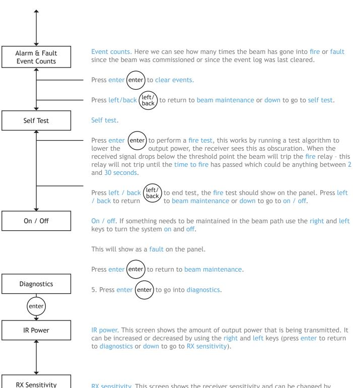
RX sensitivity. This screen shows the receiver sensitivity and can be changed by using the right and left keys (press enter to return to diagnostics or down to go to
