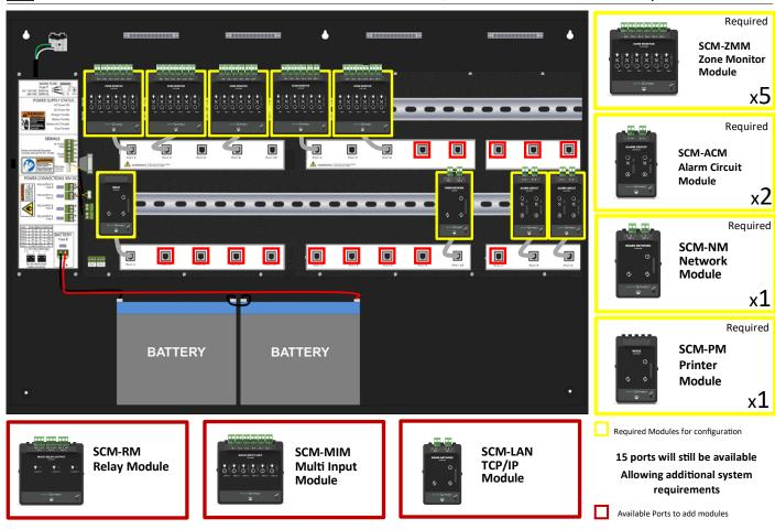
1-42 Zones with 3 x sounder circuit modules, networked & on-board printer
