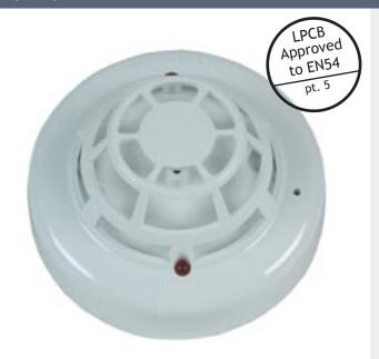
The Fyreye Class A1R (rate of rise) heat detector operates by utilising a matched pair of thermistors to sense heat. One of these thermistors is exposed to the ambient temperature, while the other is sealed inside the detector housing. Under normal conditions, both thermistors register similar readings. As fire develops, the temperature registered by the exposed thermistor will rise rapidly, resulting in an imbalance, causing the detector to go into its alarm condition.
