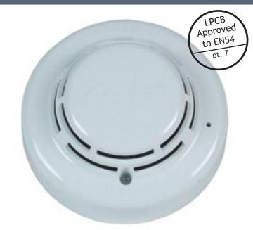
The Fyreye optical smoke detector incorporates a pulsing infra red LED Located in an optical chamber inside the detector. The chamber is designed to eliminate the effect of any external light source.
