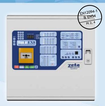
The Premier EX8 has been designed to BS EN 12094-1:2003 & EN54 parts 2 & 4 standards. It has 2 "crossed zones" for co-incidence detection for the extinguishing circuit, and 4 conventional zones for standard fire alarm detection for the rest of the installation (non-protected area).
